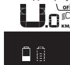
If an eBike has two batteries inserted into it and both batteries are charged on the bike, the charging progress of both batteries will be indicated on the display (the left-hand battery pack is being charged in the illustration). You can tell by the flashing indicator on the battery which of the two batteries is being charged at the moment.
